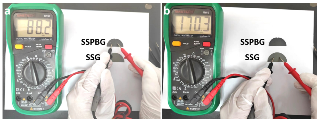
Figure S9. Photograph showing electrical conductivity of SSPBG (88.2 \Omega ) and SSG (170.3 \Omega ).
