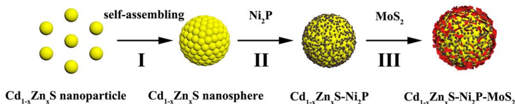
Fig. 1. Schematic illustration for the preparation of \text{Cd}_{1-x}\text{Zn}_x\text{S}-\text{Ni}_2\text{P}-\text{MoS}_2 hybrid nano-spheres
